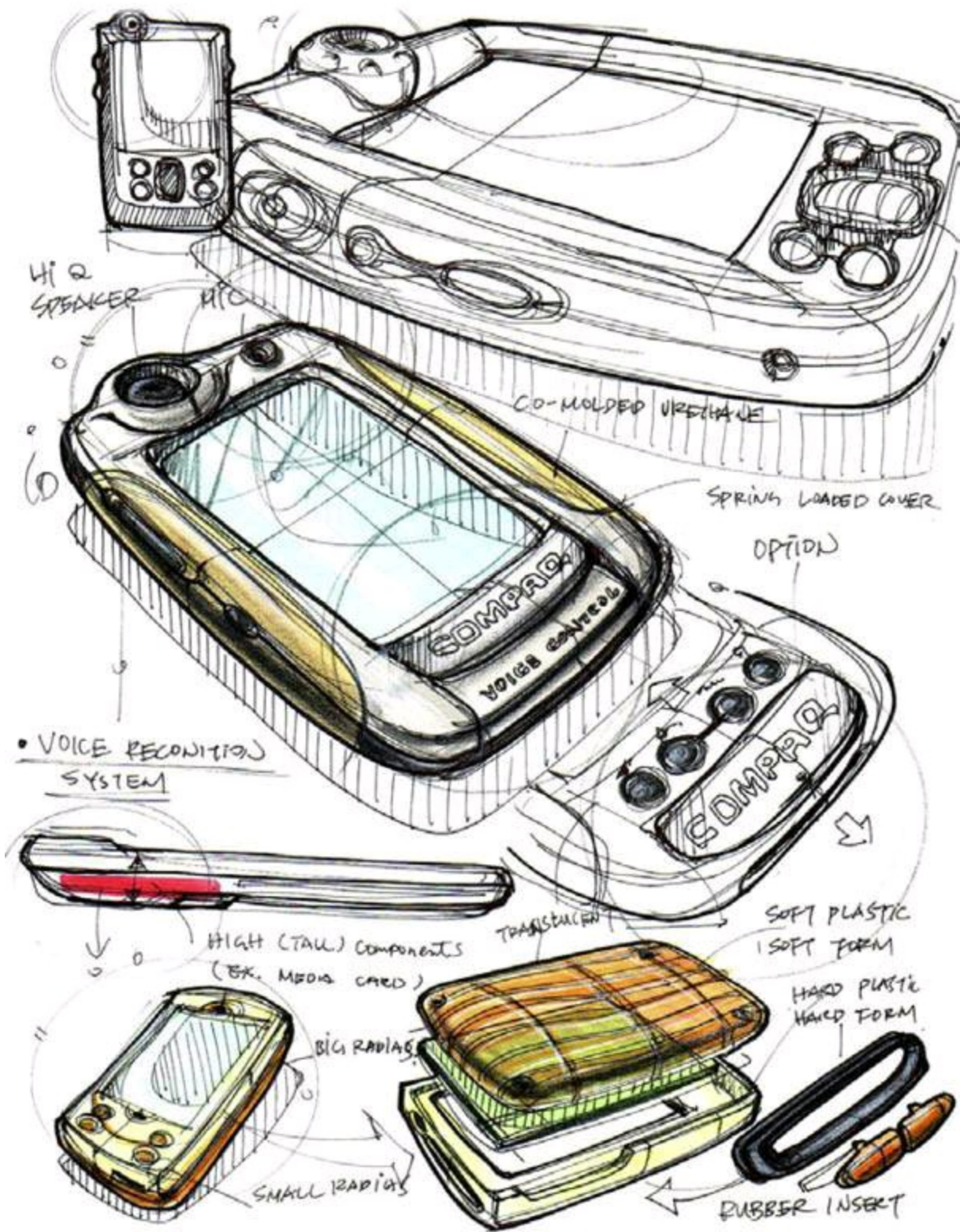
Wrapping with soft rubber for comfortable holding.
